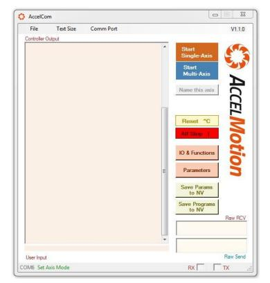
new unit is to provide a 'name' for the unit. The name acts as an address for commands and responses whenever multiple units are controlled on the same AM Comms Bus. See naming and programming chapters in your DC-series product User Guide.
