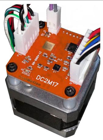
The DC2M17 is an easy-to-use compact *motor-mounted* step motor Controller/Driver, with programmable drive power, modular connectoring, and high-speed operation. It supports a wide range of motor drive parameters and step rates from ½55-step to 32,000 steps per second. Up to 52 DC-series Controller/Driver Modules can becontrolled through a fast two-wire AM Communications Bus from an external host, or can be programmed for fully autonomous operation with no external host required.
